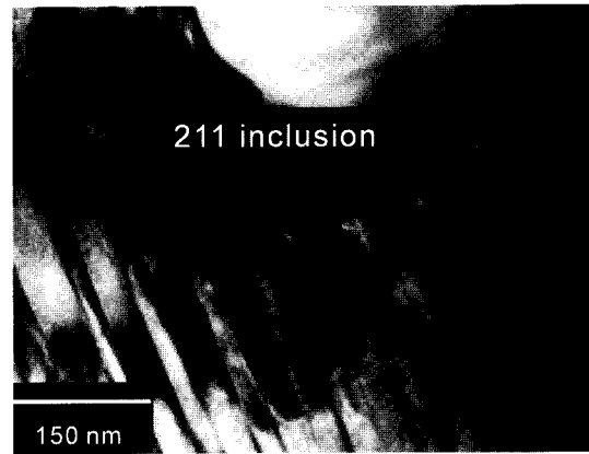
Fig. 4. TEM bright field image of the as-grown (Nd/Y)1.8 crystal showing 211 inclusions and twin boundaries.
