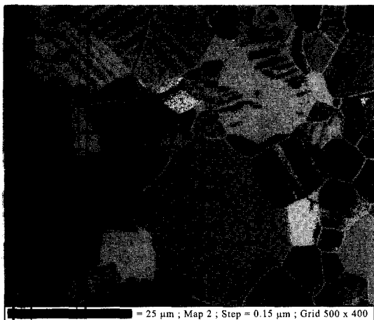
Fig. 8. EBSD orientation contrast map of \text{CaTiO}_3 .
