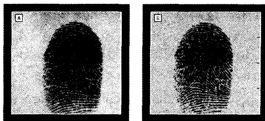
(그림 15) WSQ data-hiding 결과 ; (A)Original image (B)Reconstructed Image
