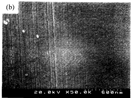
Fig. 5. (a) Friction coefficient of DLN film measured by ball-on-plate type tribometer and (b) worn surface morphology of DLN film after the wear test.
