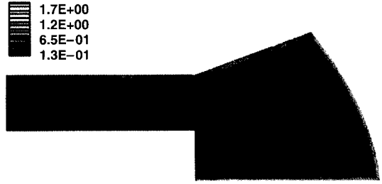
Fig. 10. Mach number contour (Injection pressure is 4 kg/cm 2 ).
