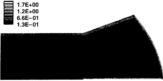
Fig. 8. Mach number contour (Injection pressure is 4 kg/cm 2 ).
