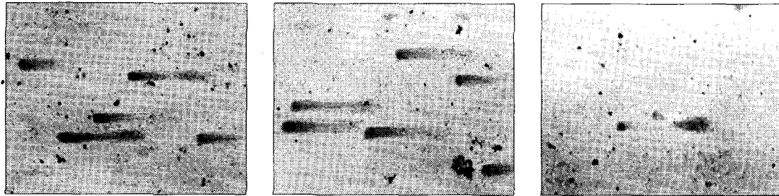
Fig. 1. DNA migration profile of orange seeds immediately after irradiation (left: non-irradiated, middle: 1 kGy, right: 2 kGy).
