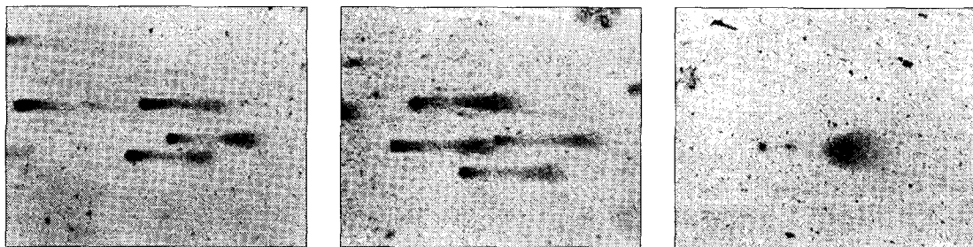
Fig. 2. DNA migration profile of orange flesh immediately after irradiation (left: non-irradiated, middle: 1 kGy, right: 2 kGy).
