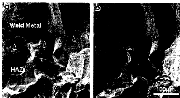
Fig. 2 Fractographs illustrating epitaxial growth of columnar grains from coarsened HAZ grains. Arrow marks represent fusion boundary (a) before etching, (b) after etching
