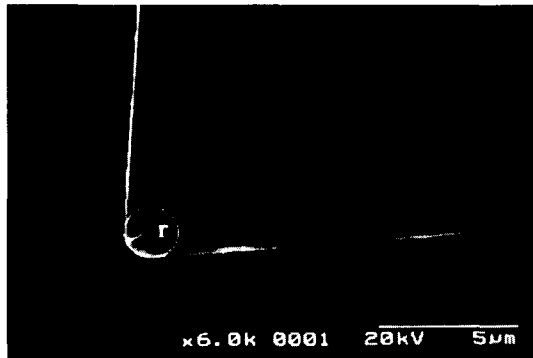
Fig. 4 SEM photograph of the diamond tool edge
