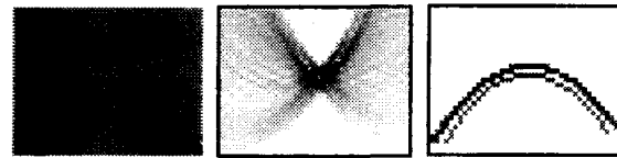
(a) Electric Line (b) Accumulator Matrix (c) Estimated Electric Line with different slope
