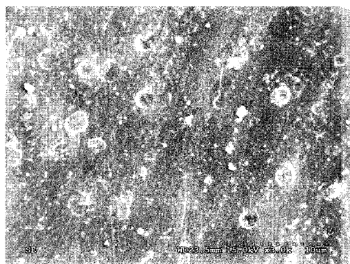
Figure 6. Dynamic mechanical values of modulus G' and G'' versus time for epoxy/PEI(10 phr) system cured at 130°C (a) and a SEM photograph (b).
