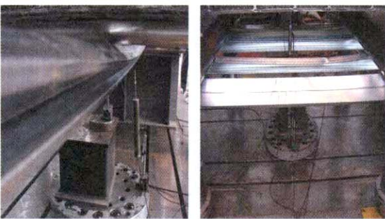
(b) 휨-비틀좌굴(Flexural/Torsional buckling)
