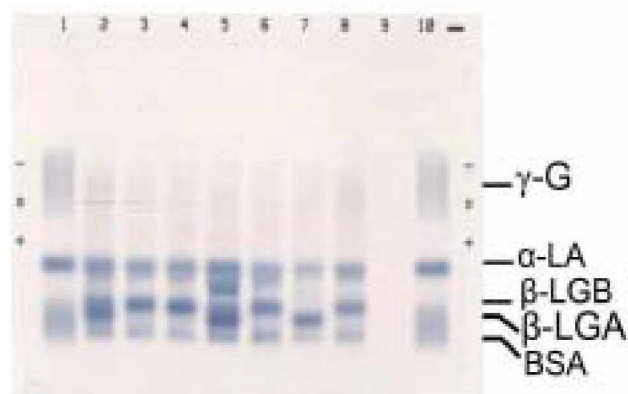
Figure 4. Electrophoresis pattern of whey proteins from Holstein cows during a humid tropical summer. Whey protein was prepared as supernatant of milk centrifuge at 10,000×g followed by acidification to pH 4.6. Electrophoresis was conducted on a commercial pre-cast agarose gel at pH 8.6, 90 mV. Lanes 1 and 10 are standards, lanes 2 to 8 are samples of representative cows.
