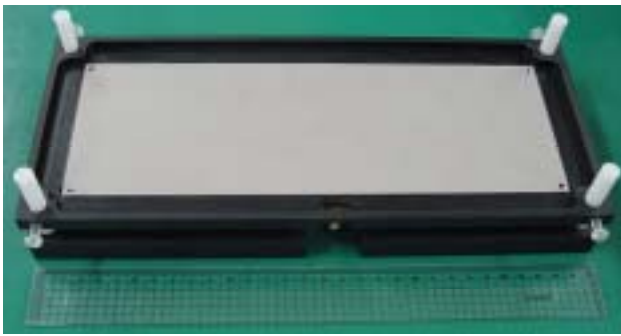
(a) Assembled antenna structure
