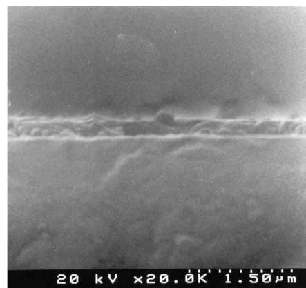
Figure 9. Side-cut view of SEM images of the ferrite/DBPA 50 layers on a glass substrate (scale bar: 1.5 \mu\text{m} ).
