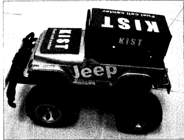
Fig. 9. A miniature car powered by a DMFC pack with a total power of 2.4W.
