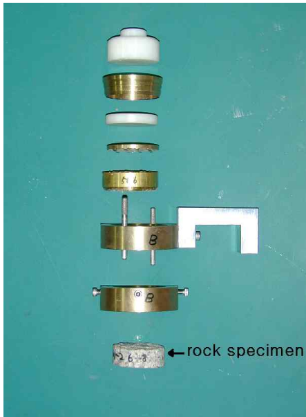
Figure 7. Assembly of direct shear box between rock and soil
