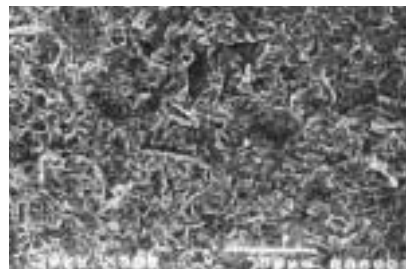
〈그림 8〉 The SEM micrograph of the specimen d (1st ; 650 → 980°C[no hold] in air, 2nd : 650 → 980°C[no hold] under vacuum,×500)
