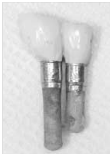
Fig. 5. Retrieved implant complex of Steri-oss system.
