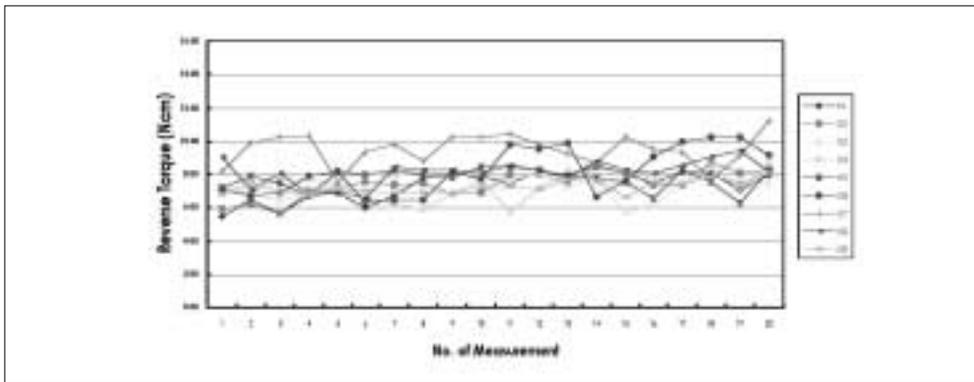
Fig. 7. Reverse torque of the group I (control group) (1-20)
