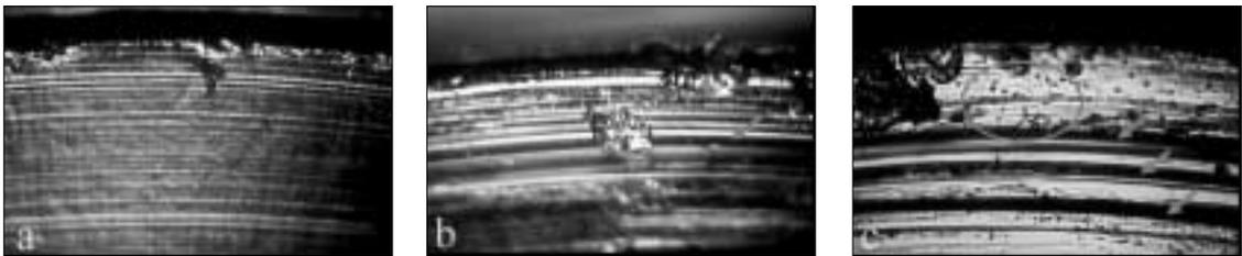
**Fig. 22.** Electroplated group (a) initial (b) after 20 measuring (c) after 100 measuring
