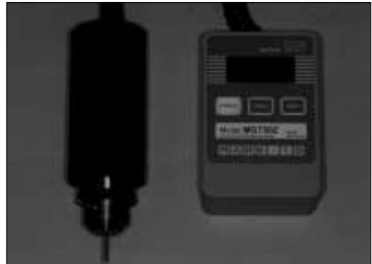
**Fig. 2.** Digital torque gauge
