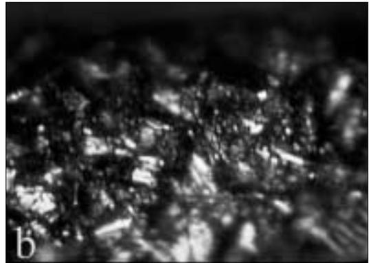
**Fig. 18.** Microphotograph of thread surface (sandblasted group) (a) X100 (b) X200
