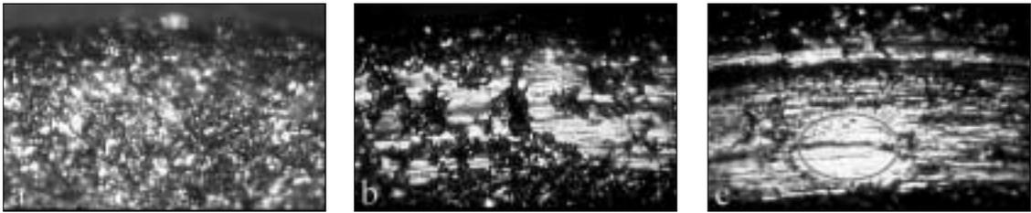
**Fig. 21.** Sandblasted group (a) initial (b) after 20 measuring (c) after 100 measuring
