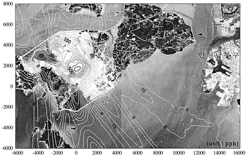
Fig. 3. The NOx weekly Concentration of Incheon Airport area by EDMS (1998.3.15~21)
