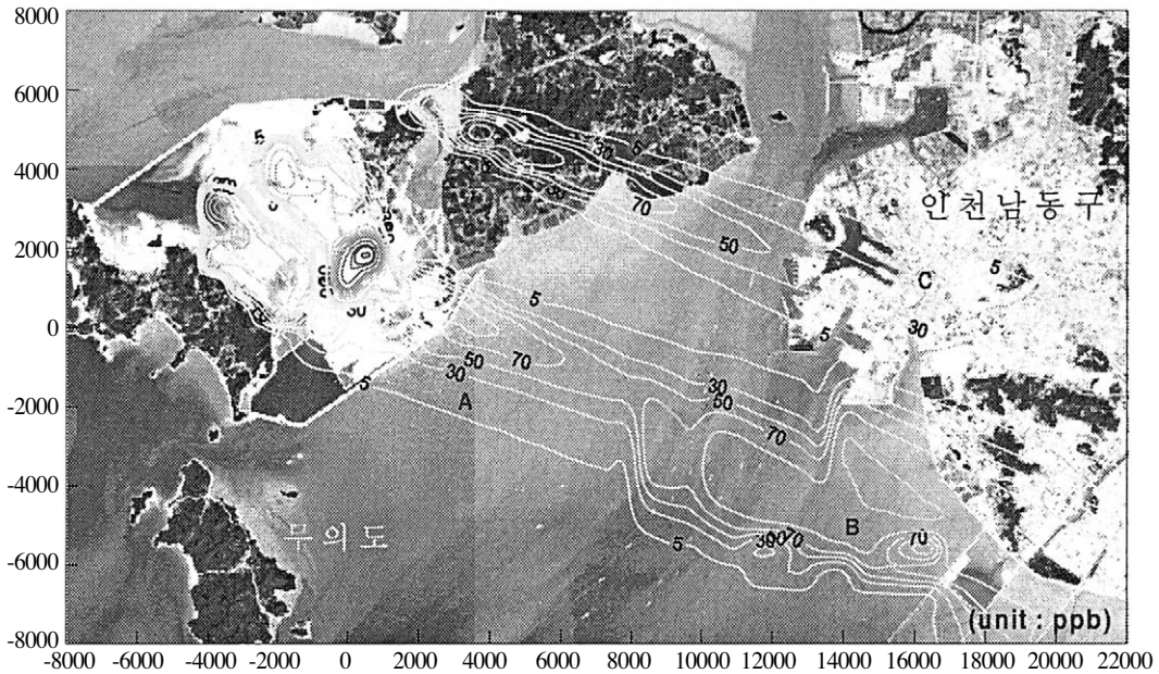
Fig. 4. The NOx hourly Concentration of Incheon Airport area by EDMS(1998. 3.15 08:00)
