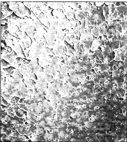
Fig. 6. SEM photograph showing fracture surface of Vertex(25KV, X30.0).
