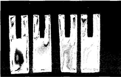
Photo. 3. c. Fringe pattern of model of type 3 in mesiodistal section.
