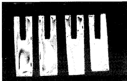
Photo. 6. c. Fringe pattern of model of type 6 in mesiodistal section.
