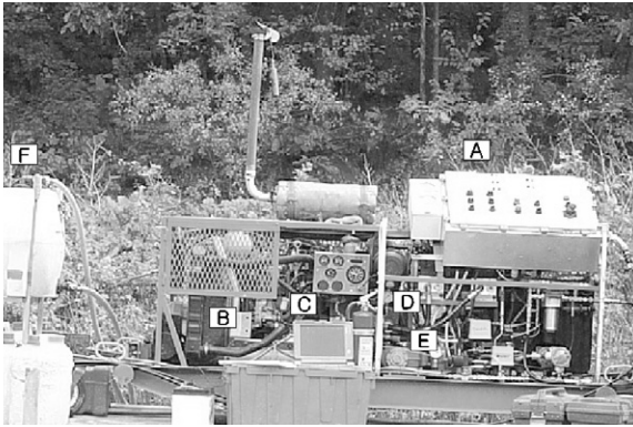
Fig. 4 A View of Some Parts of Field Measuring System A: Control Unit, B: Power Unit, C: Data Recording Unit, D: Hydraulic Pump, E: Multi-piston Water Pump, F: Water Tank
