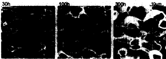
Fig. 14. Changes in microstructure of delta-pearlite during annealing at 1200°C (by SEM).
