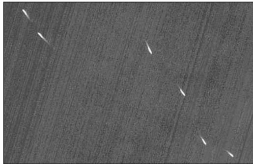
FIGURE 3. Shape of vessels on the panchromatic imagery appeared just streamline with following wave
