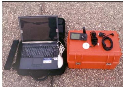
FIGURE 2. GPS equipment for data collection
