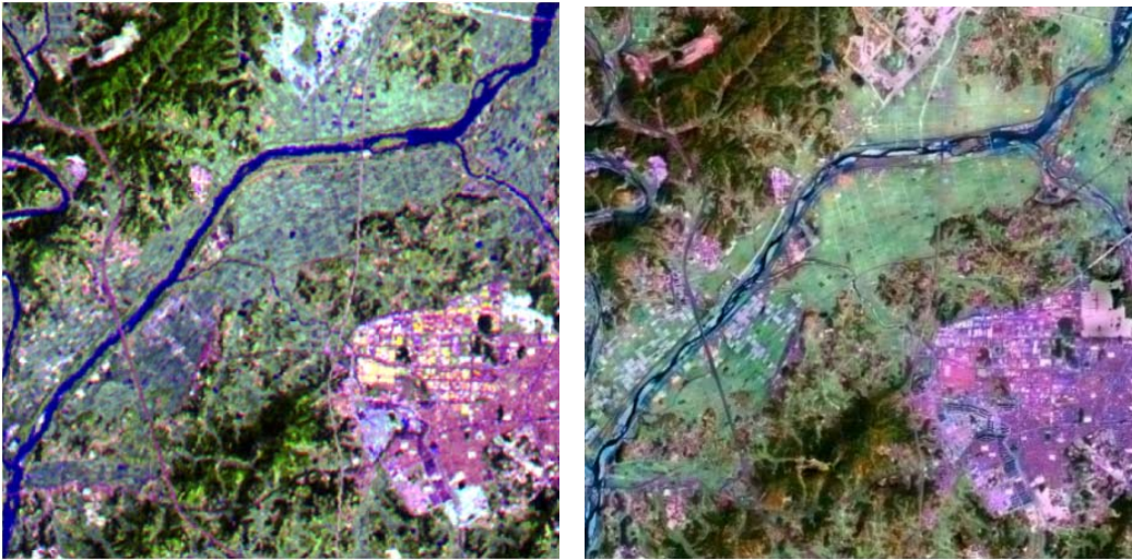
FIGURE 5. (a) Landsat TM Image of Miho river basin (b) Result of the fusion by the wavelet 6th stage
