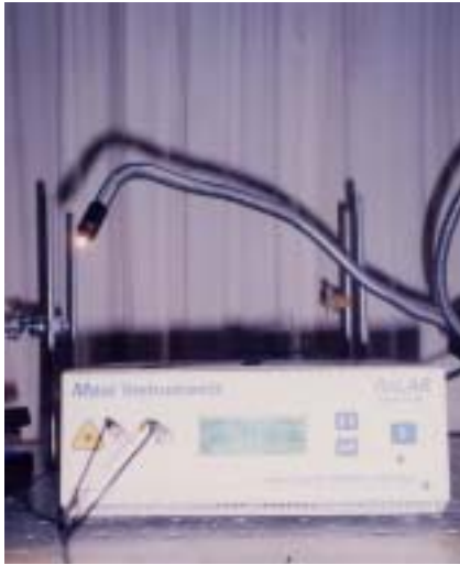
Fig. 2. Laser Doppler Flowmeter. (floLAB ® , Moor Instruments Ltd., England).
