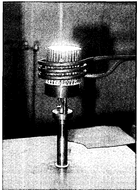
Fig. 3. A skull within RF electrical coils.
