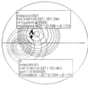
Fig. 5 Available gain and noise figure circle.
