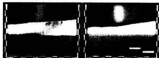
Figure 5. Infiltration behaviors of seawater (left) and fuel oil C (right) by wave and tidal actions after 1,500 sec.
