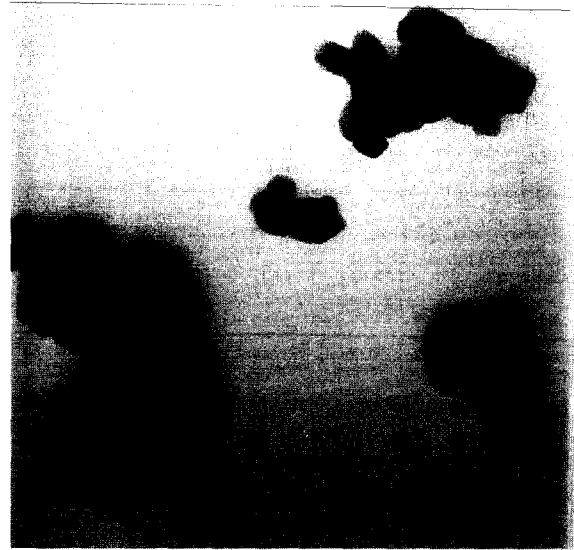
Fig. 3. TEM micrograph of the synthesized CeO 2 nano-particles, which shows aggregate structures of less than 100 nm in size.
