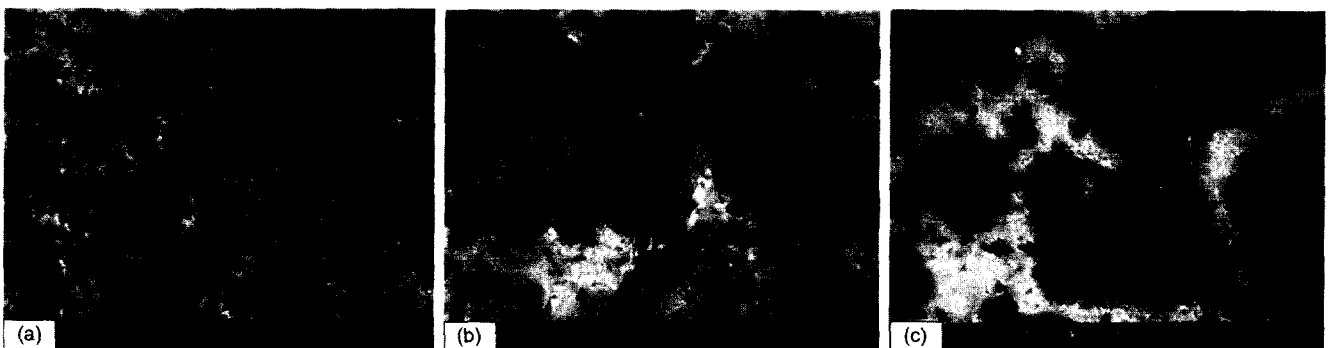
Fig. 4. SEM pictures of B 4 C/Al cermet prepared by: (a) infiltration at 1100°C/10 min in vacuum and then followed by post-heat treatment at 900°C for (b) 4 h and (c) 8 h.
