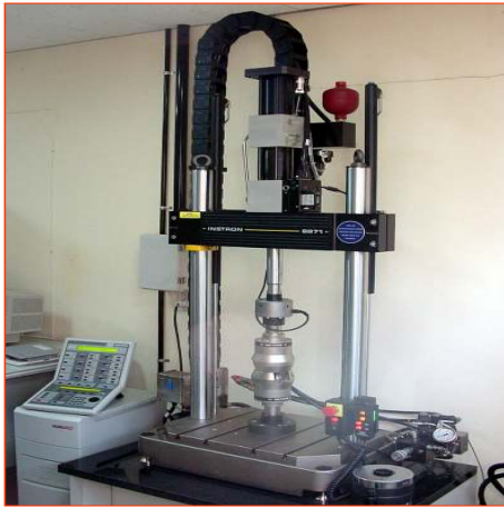
Fig 6. Universal test machine (Instron 8871 ® )
