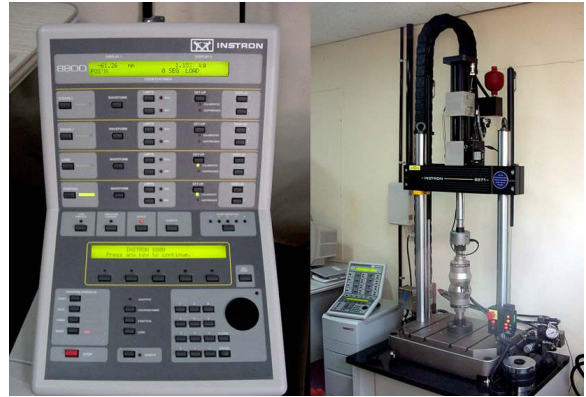
Fig. 5. Loading machine (Instron 8871, Instron Corporation, U.S.A.)
