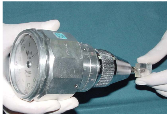
Fig. 8. Measuring loosening torque
