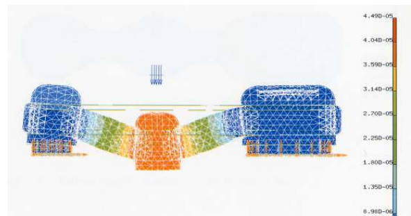
Fig. 6. Displacement in the bridge of band. Max. vertical displacement of approx. 0.045 mm
