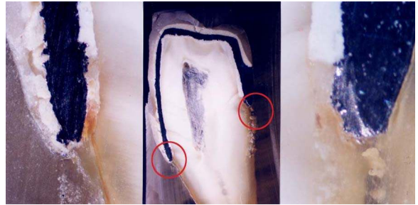
Fig. 4. Magnification(*70) of buccal & lingual margins on block sectioned specimen of premolar tooth(*10)
