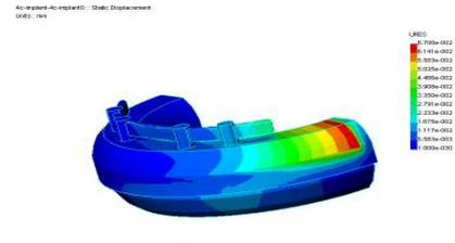
Fig. 48. OVD4-can (90°): Displacement
