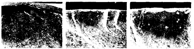
Fig. 11. SEM photographs of fracture surface around crack initiation point (SUP 7 under 2 stage shot-peened).
