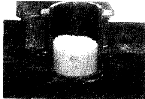
Fig. 4 Settlement of cellular concrete
