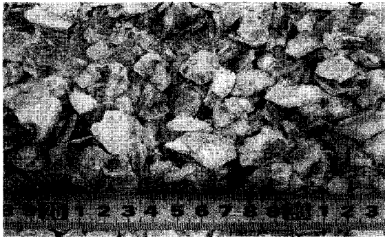
Fig. 4 Grading of crushed oyster shells as coarse aggregate
