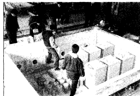
Photo 2 Heater for test of fire resistance
