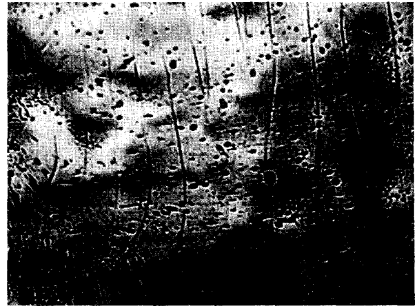
Fig. 9. Magnetic domain pattern of Fe_{72}B_{14.4}Si_{9.6}Nb_4 amorphous alloy with the thickness of 22 \mu m which was annealed at 500 ^{\circ}C for 20 min ( \times 100 ).
