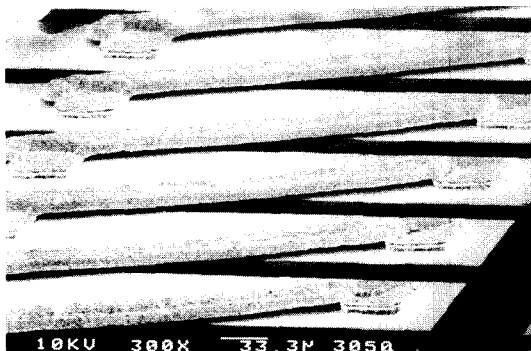
Fig. 10. The SEM photograph after fabrication of air-bridge.
