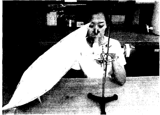
Fig. 2. The apparatus for collecting exhaled a breath sample from each subject. The subject was asked to close her nose with a clip and breathe (inhale and exhale) via the mouth only. She inhaled air purified through the filter and exhaled breath into the 15 L non-diffusing sampling bag. The collected breath was transferred into an adsorbent tube filled with Tenax TA (20/35 mesh, 70 mg) and Carboxen 569 (20/45 mesh, 130 mg).
