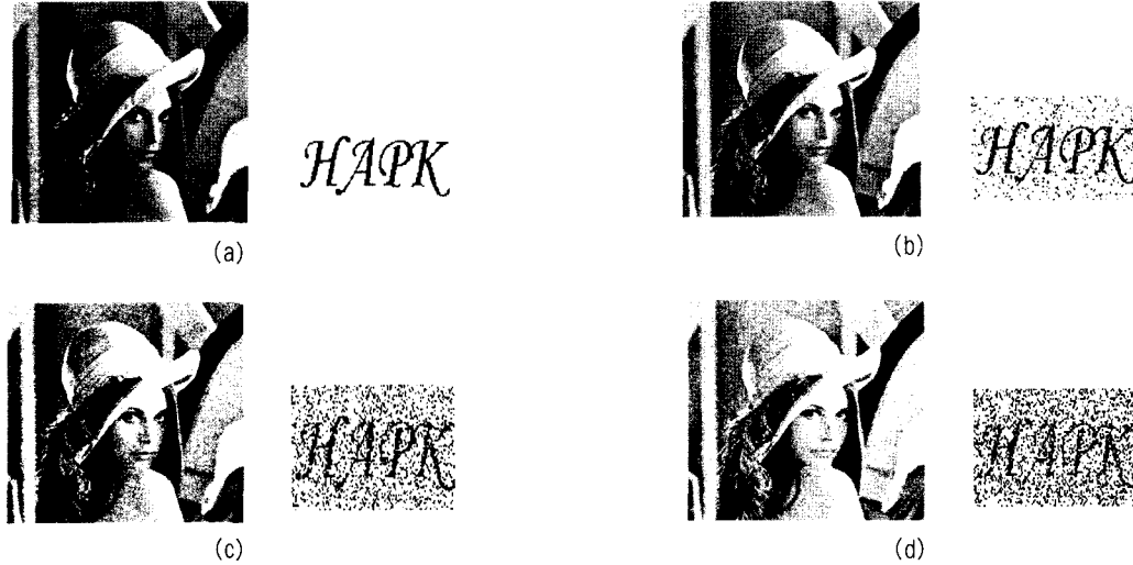
Fig. 9. The message retrieved from the stego-image "Lena" under Gaussian noise with different noise (a)Gaussian noise, \beta = 20\% (NC=1.0000) (b)Gaussian noise, \beta = 30\% (NC=0.9194) (c)Gaussian noise, \beta = 40\% (NC=0.8018) (d)Gaussian noise, \beta = 50\% (NC=0.7462)
