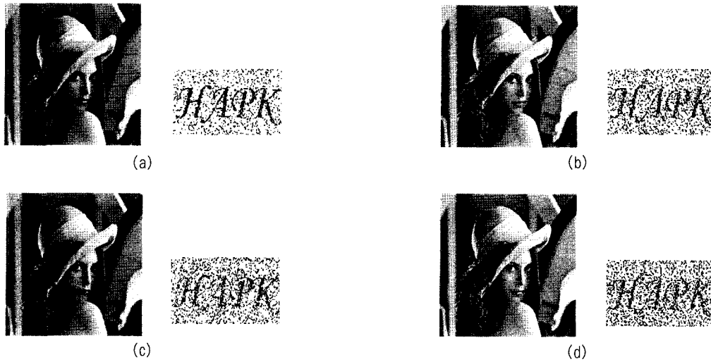
Fig.7 The message retrieved from the sego-image "Lena" after JPEG compression with different compression ratio. (a)JPEG Compression ratio=17.71 (NC=0.8633) (b) JPEG compression ratio=18.18 (NC=0.8053) (c)JPEG compression ratio=19.69 (NC=0.7862) (d) JPEG compression ratio=23.69 (NC=0.7862)
