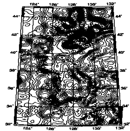
Fig. 10. The difference of geoid undulations between EGM96 and GPM98A up to degree and order 720 (C.I.:10cm).
