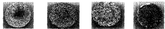
(a) T = 585\text{ }^\circ\text{C} (b) T = 595\text{ }^\circ\text{C} (c) T = 615\text{ }^\circ\text{C} (d) T = 680\text{ }^\circ\text{C} d_{avg} = 0.839mm d_{avg} = 1.189mm d_{avg} = 1.341mm d_{avg} = 2.740mm
