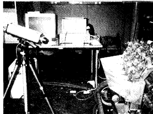
Fig. 3 Vibration measurement of the metering device using a laser-based vibrometer.
