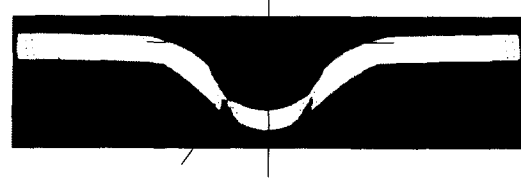
Fig. 5 A cross section of SP-creep with creep time, 84hrs at 600 °C
